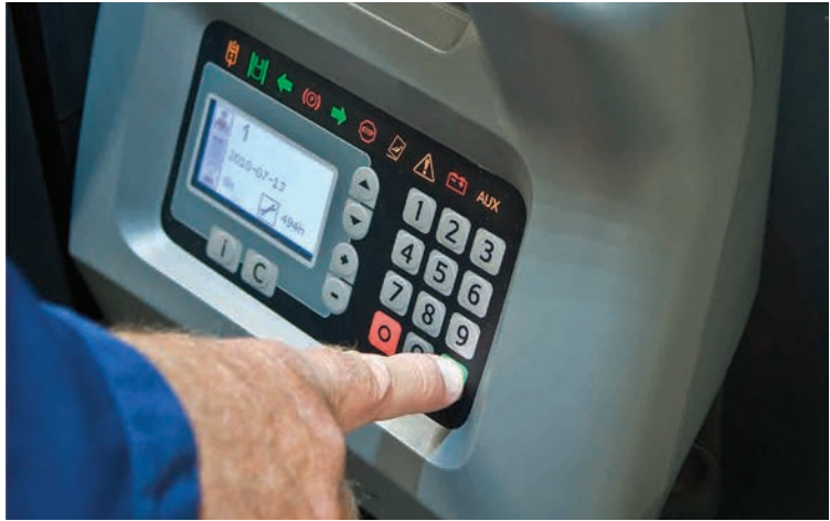
BT Access Control prevents unauthorised use and preset each driver's personal parameters upon start-up
