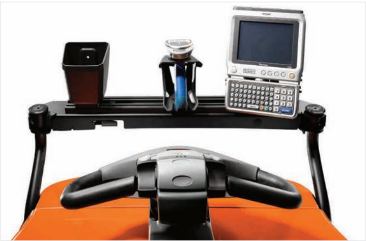
Optional powered E-bar allows easy mounting of ancillary equipment
