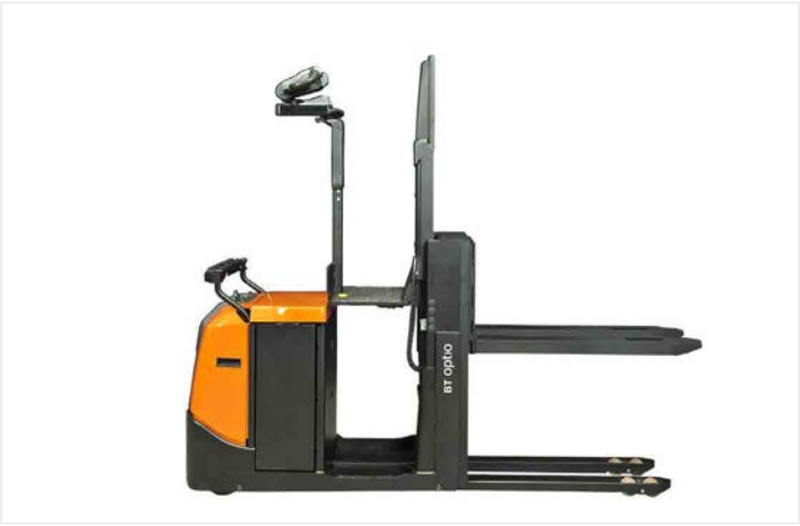
Several models feature platform lift for picking at the second level
