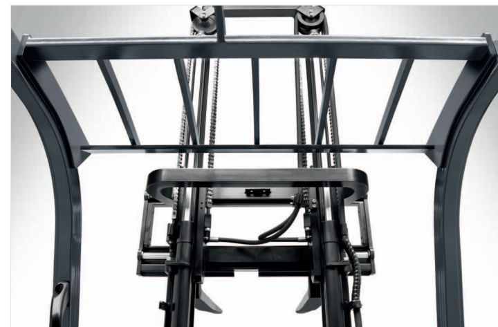
Visibility FV mast provides a clear view at all angles
