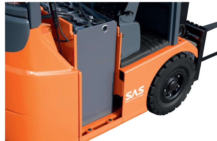
Standard low lift-out battery extraction. Optional built-in rollerbed for fast changes
