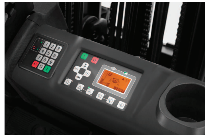
Multifunction display gives key information at a glance, as well as allowing the parameter settings to be adjusted to suit the needs of the application
