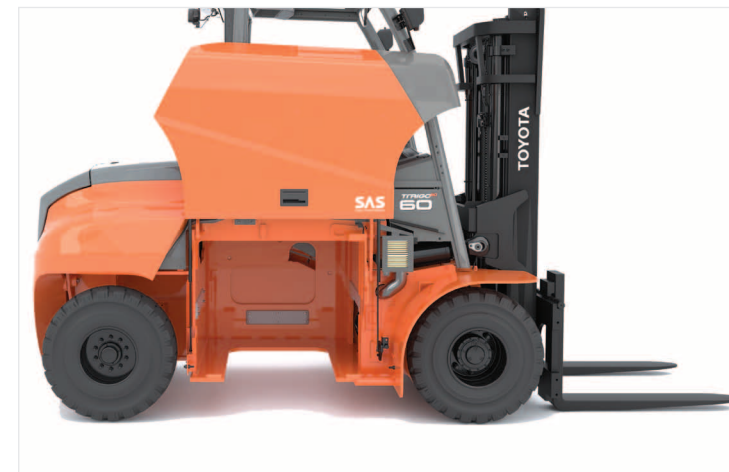
Open chassis design with side panel facilitates lateral battery exchange.
