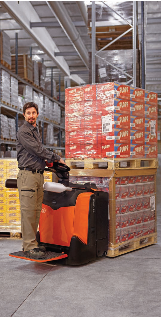
The height of the steering arm can be adjusted at the touch of a button
