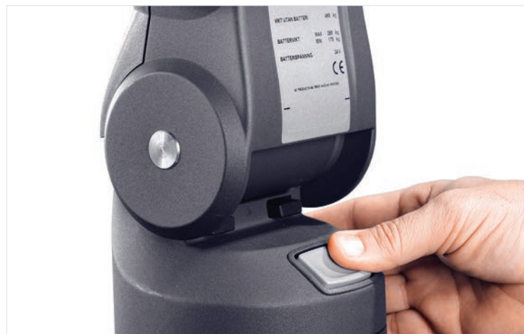
One-touch action to adjust the height of the tiller arm
