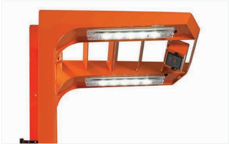
Overhead guard with integral LED working lights
