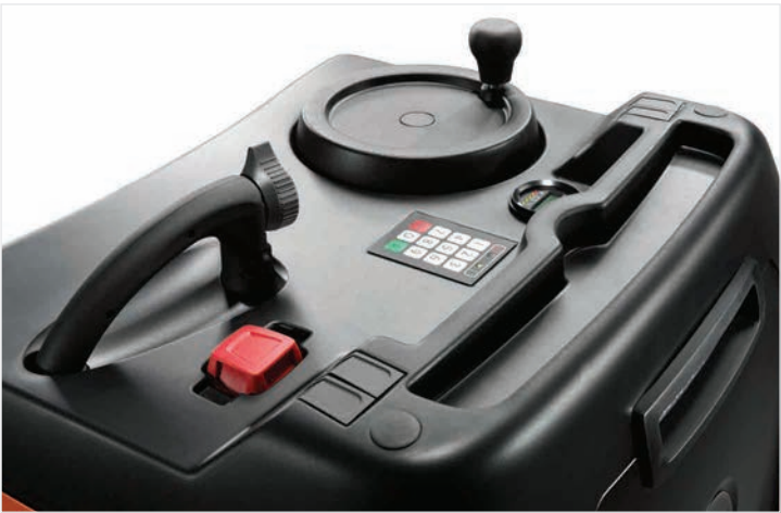
Spinner wheel' steering and PIN-code access
